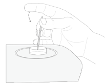
Figure 3. Cover the open end of the straw with index finger
